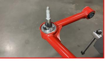
Install the provided upper control arm dust cap. Ensure the "R'' is facing towards the outside of the vehicle.
