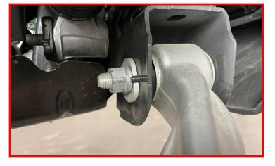
Tighten the (3) top strut nuts. Torque the M10 nut to 35 ft-lbs.
