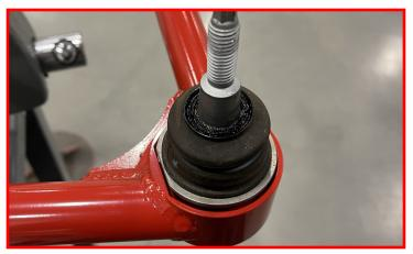
Install the factory ball joint retaining clip.
