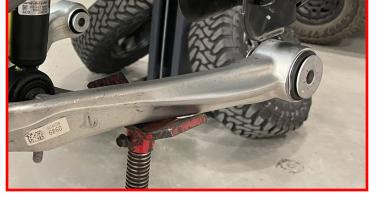
Install the factory alignment cam plate over pivot bolt and then install nut.
