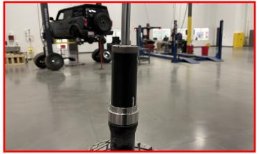
Install the lower strut coil perch. Ensure the mark made in the previous step is aligned in the factory orientation.
