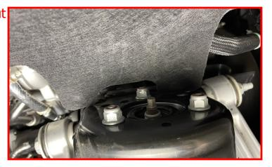
Remove the lower strut nuts.
