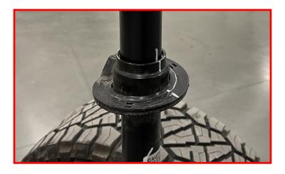
Install the seal head bump cap.
