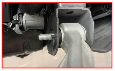
With the lower control arm pivots removed from the frame pockets, Swing the lower control arm down while removing the lower strut studs from the control arm.
