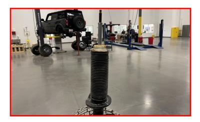
Remove the seal head bump cap.
