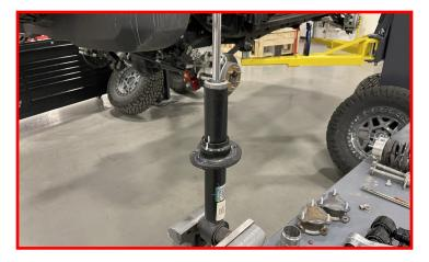
Install the seal head bump cap.
