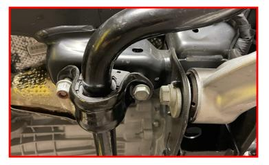
Torque the factory nut to 55 ft-lbs. Torque the factory bolt to 55 ft-lbs.
