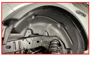
Remove the rear fender liners.
