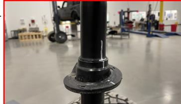
Install the preload collar over the strut body. Ensure the collar is completely seated on the retainer clip.
