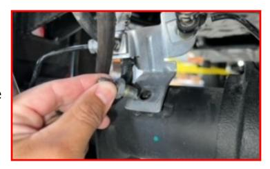
Remove the shocks on both sides of the vehicle.
