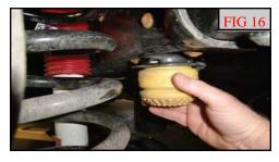
Remove the factory bump stop by pulling it out of its mount. Remove the mount from the frame. (Fig 16)
