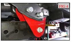
Install the ReadyLIFT® radius arm drop brackets into the frame using M18 x 130mm bolts, washers, crush sleeve, and nuts. Do not tighten at this time. (Fig 3)
