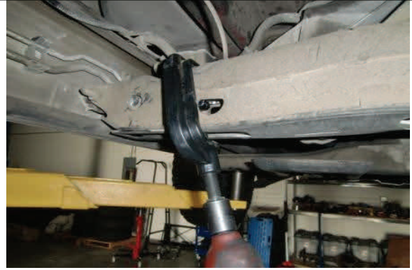
Reinstall tool and adjust upward enough to insert adj. block
