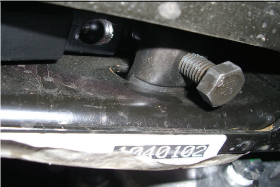
Install new adj. bolt and make bolt flush with cross-member
