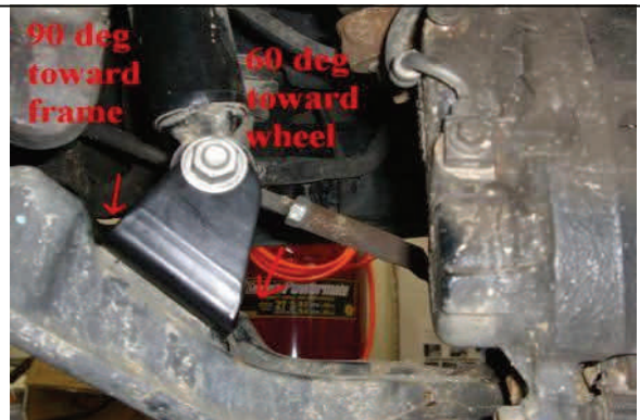
Install new extension bracket with OE bolts as shown
