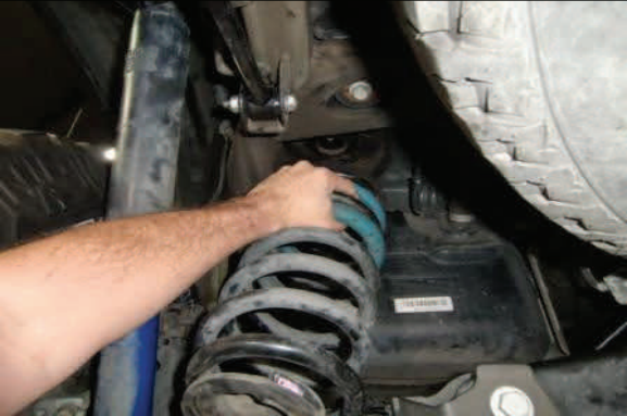
Carefully lower axle and remove coil springs and isolators
