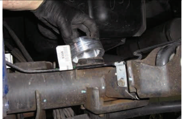
Place ReadyLIFT spacer on axle mount
