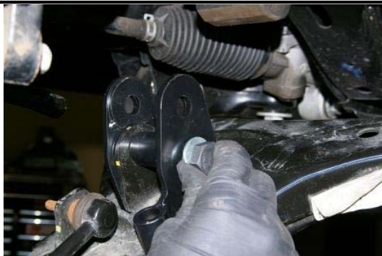
7. Remove the three upper strut mounting nuts, lower mounting bolt, and remove the strut.
