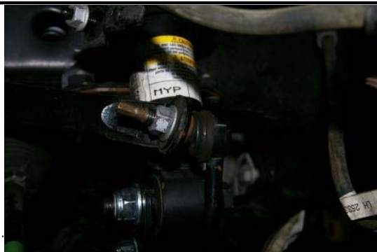
10. Install the M12 bolt, two washers, and c-lock nut. Do not tighten.
