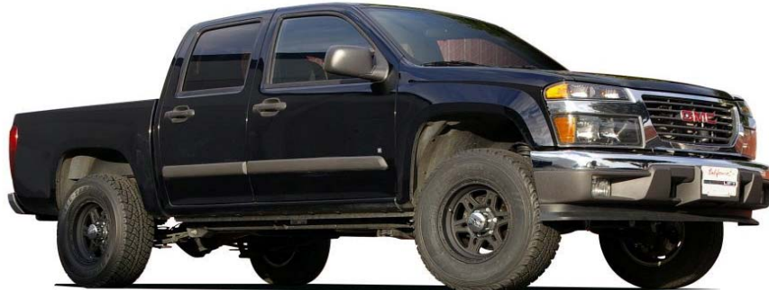
After ReadyLift® 69-3075 SST Kit. Raceline Renegade 6 wheels 16x8 0 offset on 255/70R16 All-Terrain Tires
