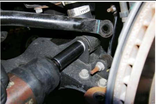
3. Unbolt the 15mm upper sway bar end link nut. Separate end link from sway bar.
