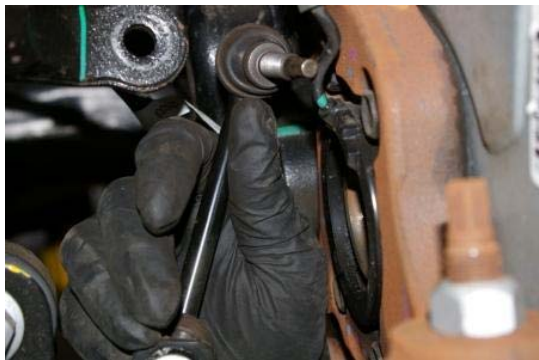
1. Remove the front wheels. Unclip the ABS line from the upper control arm.
