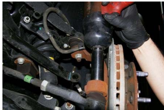
2. Unbolt the 13mm ABS line retaining bracket nut.
