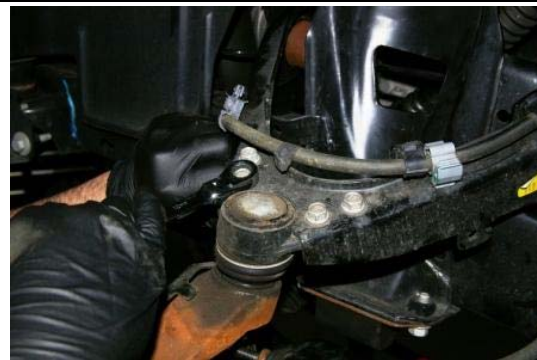
4. Unbolt the 21mm tie rod end nut. Separate the tie rod end from the steering knuckle.
