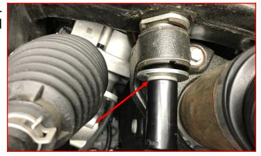
Mounting bolts are located between the rack and the CV axles on both the driver and passenger sides.
