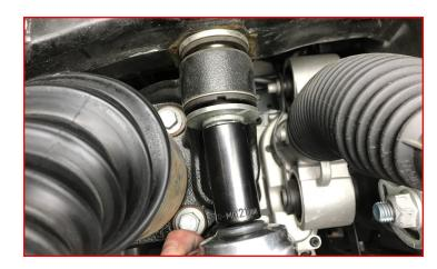
Slide diff drop retainer plates in between factory diff mounts and frame rail. Install supplied M14 bolt, washer into frame a few turns, Enough to start the threads. Do not tighten at this time
