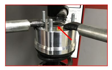
Install factory washer and supplied M10 Flange nut to shock shaft, tighten and torque to 30-ft./lbs.
