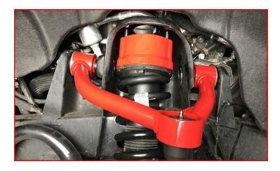
Raise the lower control arm up and install the lower strut mount using factory hardware. Do not tighten at this time.
