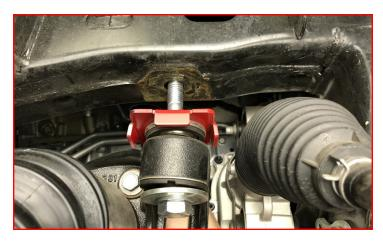
Install diff drop spacers between diff drop retainer and the differential mount.
