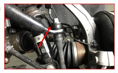
Loosen but do not remove axle nut. Press axle back through hub to allow for greater misalignment and ease in the removal/installation process.
