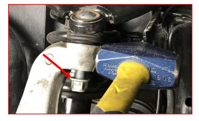
Support the lower control arm with a suitable jack. Remove the lower strut mounting bolt from the lower control arm.
