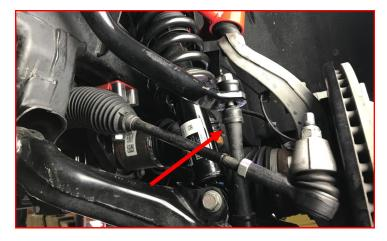
Install brake line bracket spacer using the factory hardware. Align bracket to match angle of the upper control arm and tighten.
