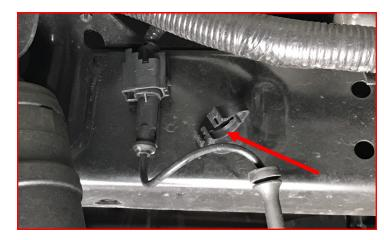
Driver side: Open the clip and remove the ABS wire.
