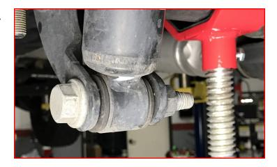
Install the rear wheels and lower vehicle to the ground. Torque the lug nuts to the wheel manufacturer specs, the lower shock hardware to 45-ft/lbs and u-bolts to 110-ft/lbs. Attach the vehicle negative power source. Have the alignment set to the recommended specs at the end of the instructions.
