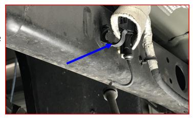
Support the axle with a suitable jack. Remove both Driver and Passenger shock bolts from the axle.
