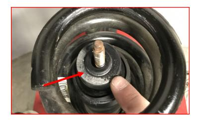
Install supplied shock bushing crush sleeve to shock shaft.
