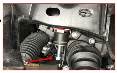
Release support from differential allowing the diff mounts to slide down mounting hardware. The differential may need a little assistance sliding down to the head of the bolt.
