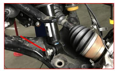
Install the upper ball joint to the knuckle using provided hardware.
