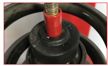
Install the replacement top hat and the rubber isolator taking care to install in same orientation as the factory top hat.
