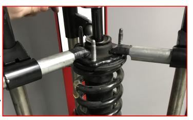
Install supplied shock bushing half to shock shaft.
