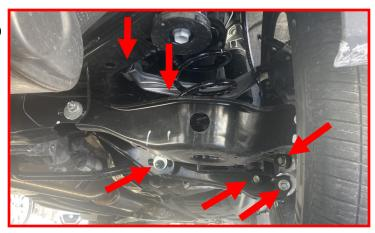
Once you've loosened the components on both sides of the vehicle, roll the vehicle back and forth a few times to let the suspension free itself.
