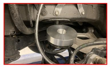
Once complete, position the spring spacer into the factory spring locator.
