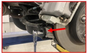
Loosen but do not remove the inner eccentric bolt.
