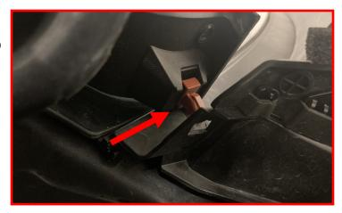
Locate the x7 plastic clips holding the cowl to the body. Remove all the clips and set aside. Gently lift up on cowling from the engine bay side, while lifting pull towards the front of the vehicle to disengage from the windshield. Once disengaged from the windshield, set aside in the engine bay.
