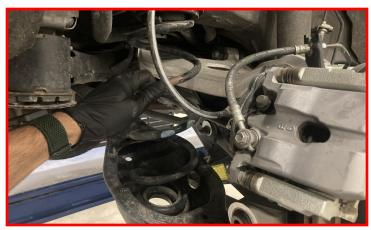
When you have enough room, place the provided spring spacer into the factory isolator.
