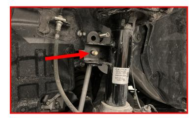
Install the factory sway bar end link to the bracket using the factory hardware.
