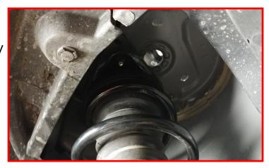
Install the provided strut spacer onto the strut mount using the factory hardware. This is a tight fit to get the strut spacer and bolts into place. Use of a pry bar may be needed for placement of the strut spacer. The top hat can be rotated to access the bolts. Once all have been started, tighten all down.
