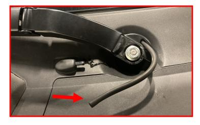
Remove the factory mounting nut. Mark the windshield wiper location against the shaft for reinstallation. Gently lift up on the wiper arm while slightly twisting. The arm should pop off the shaft.
