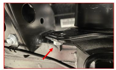
Compress the factory airbag enough to slide the ReadyLIFT rear airbag spacer between the airbag and the axle.
