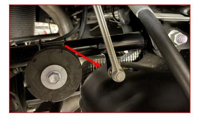
Using the supplied M6 bolt, washers, and locking nut, install the airbag ride height sensor bracket to the control arm with the bent location tab facing to the rear of the vehicle.
