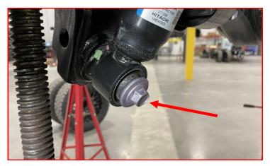
Install the rear brake line spacer between the brake line and the axle using the factory bolt (one on each side) holding the brake line to the axle.
