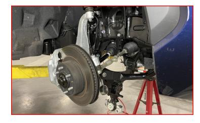
Using a suitable spring compressor, compress the strut enough to rotate the lower strut. With the Ready LIFT front strut spacer placed on top of the strut, rotate the lower strut mounting hole to be parallel to the two engraved dots on the top of the Ready LIFT front strut spacer.
