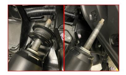
Apply a small amount of thread locker to the factory shock and install the ReadyLIFT rear strut extension onto the factory strut.
