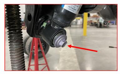
Remove the three bolts holding the factory bump stop to the frame.
