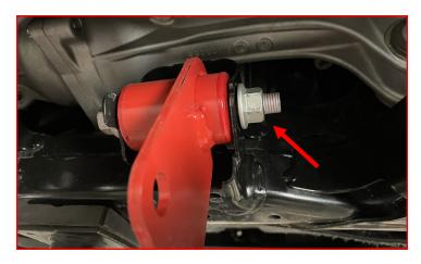
Attach the diff drop bracket to the differential using factory hardware, supplied M16 flat washers, and M16-1.5 C-lock nuts. Note the orientation of the hardware.
