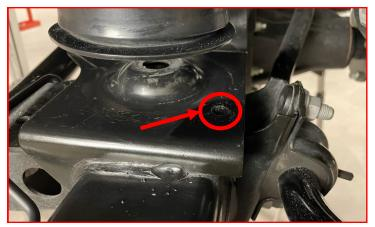
Insert the ReadyLIFT rear airbag spacer. Line the center of the spacer up with the marked location on the axle mount and factory airbag.
