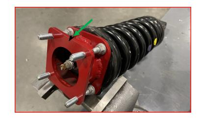
Place the strut and spacer assembly into the control arm.
