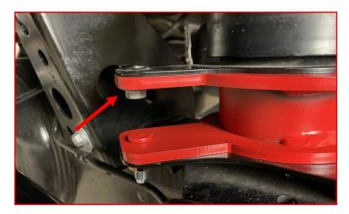
Remove the nut on the ride height sensor arm at the lower control arm.
