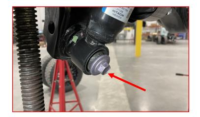
Remove the upper shock nut and bushing.
