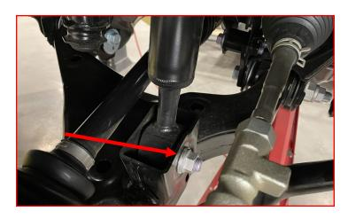
Remove the four (4) upper strut bolts.
