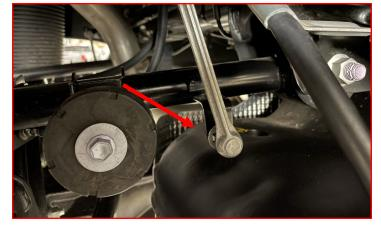
Using the supplied M6 bolt, washers, and locking nut, install the airbag ride height sensor bracket to the control arm with the bent location tab facing to the front of the vehicle.
