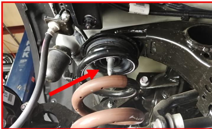
Unscrew the nut until it reaches the end of the stud. Do not fully remove. Do this for both sides of the vehicle.
