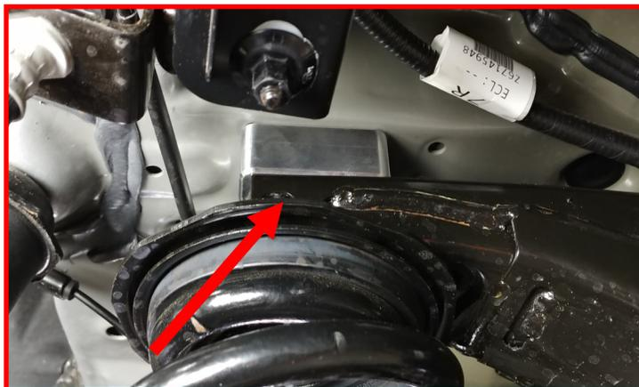
Install the round spacer in between the cradle and frame using the provided **M14 bolts, washers, and large laser cut washer**. Add a drop of thread locker to the threads of the bolt. Once all spacers are installed, raise the cradle up into place using the jack. Torque all hardware to **65 ft-lbs**.
