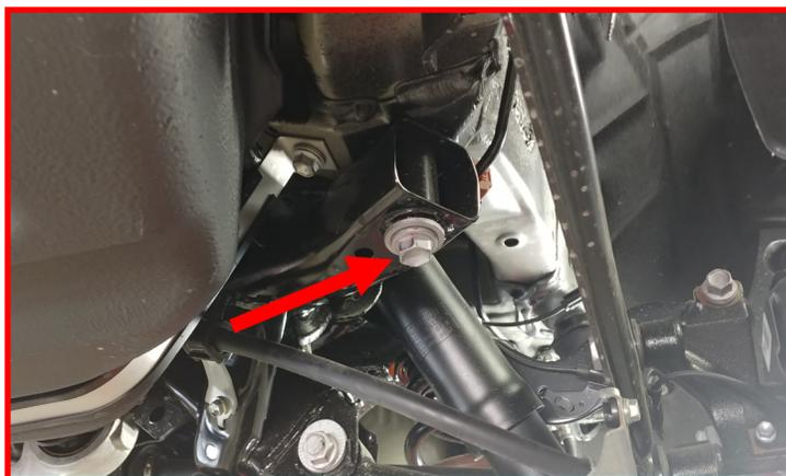
Locate the ReadyLIFT cradle spacers. The round will go in the front location and the square slotted spacers will go in the rear location above the springs.
