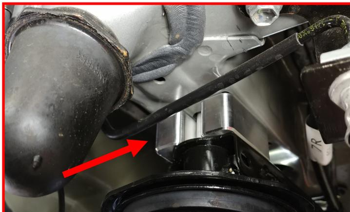
The side edges will line up with the cradle tubing as shown. Do not tighten at this time.
