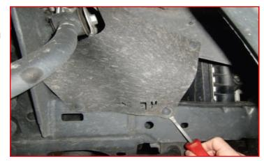
Remove the upper control arm from the frame. Take care as the upper control arm bolt is very long and has to pass through the engine compartment by some electrical harness and coolant lines. It is best to remove the lines off the inner fender well on the passenger side to gain enough access to pass the bolt forward. (Strut shown removed for clarification. Will be removed in a later step.)
