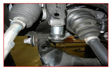
Notch the lower control arm strut pocket as shown using a suitable cutting device. Sand any burs off the cut edge. Paint the cut area with a quality rust preventative paint.
