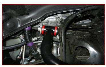
Install the upper ball joint to the knuckle using the supplied ball joint nut. Torque to 85 ft-lbs.
