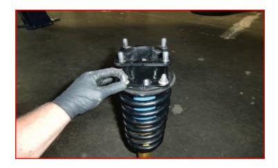
Install the completed strut assemblies into their corresponding sides using the supplied 10mm nuts. Do not tighten at this time. It may be easier to only install the nuts closest to the engine bay finger tight so that the struts have some wiggle room to move around while lining up the lower strut bolts. Raise the lower control arm into place and install the lower strut using the factory hardware. Do not tighten at this time.
