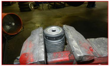
Use a suitable cutting device, remove the tip of the shock shaft right above the first thread. Sand any burs off.
