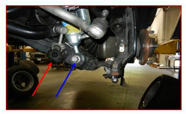
Remove the lower ball joint cradle bolts. Loosen but do not remove the lower control to frame bolts. Let the lower control arm swing out of the way. Remove the strut from the upper frame mount.
