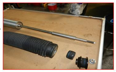
Stretch the boot until it fits over the shock body and install the hose clamp to hold boot in place.
