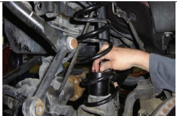
Install new springs/bumpstops extensions simultaneously.
