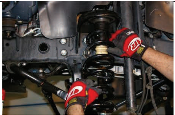
Carefully lower front axle enough to remove front springs.
