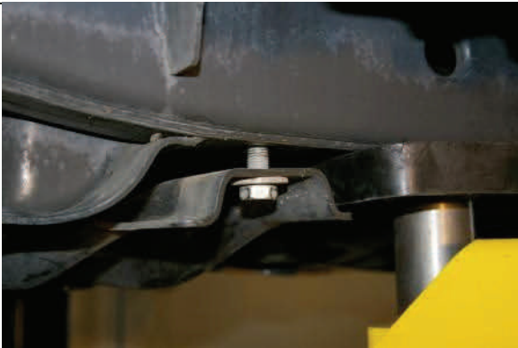
Remove (2) front transfer case skid plate bolts.
