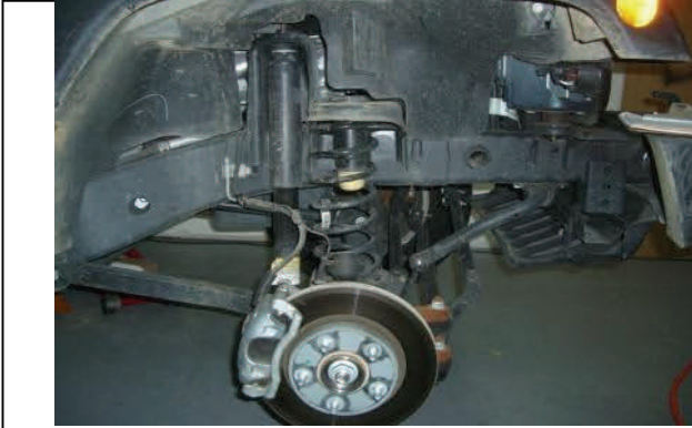
Securely raise vehicle off ground and remove (4) wheels
