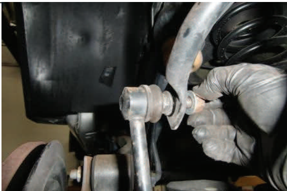
Disconnect and remove rear swaybar endlinks
