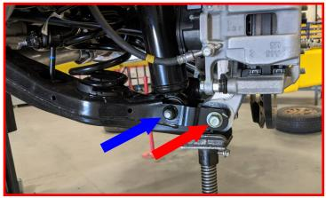
Install the sway bar end links to the lower control arms using the factory hardware torque to 40ft-lbs.
