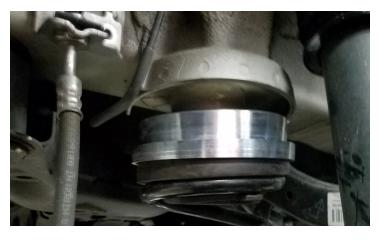
Seat the spring on the lower spring seat. Ensure that the spring is seated correctly against the stop on the lower spring seat.
