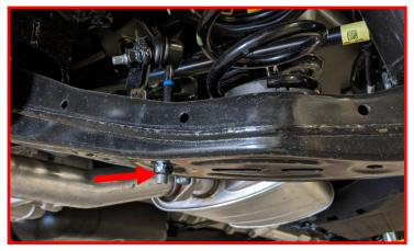
Loosen but do not remove the rear alignment cam bolts.
