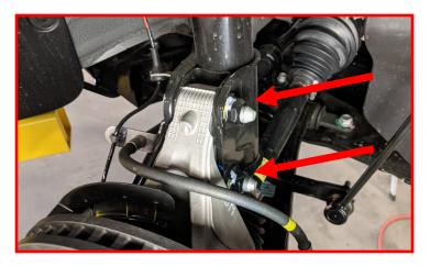
Reattach the ABS and brake line bracket to the strut body.
