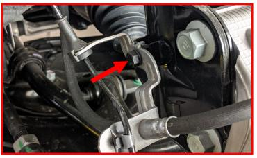
With an adjustable jack under the lower control arm, remove the strut to knuckle fasteners. Retain factory hardware.
