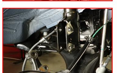
Locate the ReadyLIFT front strut extension. Install to the top of the strut using the factory hardware. Torque to 30 ft-lbs. Set assembly aside and move on to next step.
