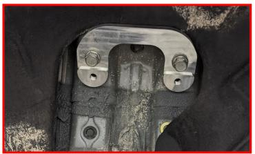
Using the supplied M12x35mm bolts and washers, install the shock into the lower shock extension. Torque to 50 ft-lbs.
