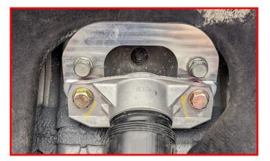
Add the ReadyLIFT spring spacer to the top of the spring. Use the rubber isolator between the spring and spacer.
