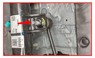
Remove the brake line bracket and ABS wire at the strut body. Let hang out of the way. Retain factory hardware.
