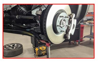
Remove the factory sway bar end link from the strut assembly. Retain factory hardware.
