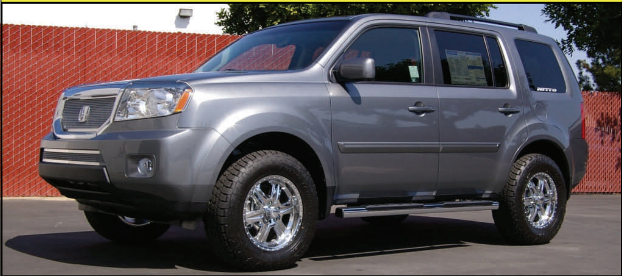
After ReadyLift® 69-8020 SST Lift kit. 265/65R17 Nitto Terra Grapplers on 17x8.5 +30 offset AR Fuel. Minor trimming needed.
