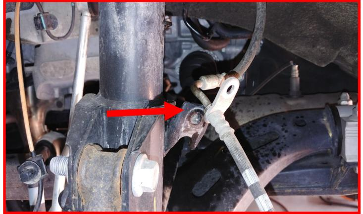
Remove the **ABS harness clip** at the strut body. Let hang out of the way. Remove the strut to **knuckle bolts**. The bolts are specific to upper and lower mounting locations and direction of install. The upper is a cam bolt, while the lower is a standard bolt. Make sure to note their orientation for reinstallation later.
