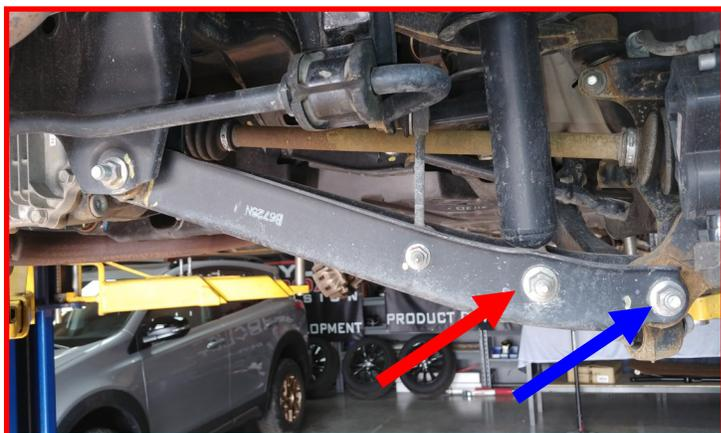
Install the lower front control arm to the knuckle using the **factory hardware**. Do not tighten at this time.
