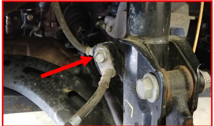
Install the ReadyLIFT sway bar bracket to the strut using the provided **M12 bolts, washers, and nuts**. Install the factory end link to the ReadyLIFT bracket using the **factory hardware**. Torque all to **45 ft-lbs**.
