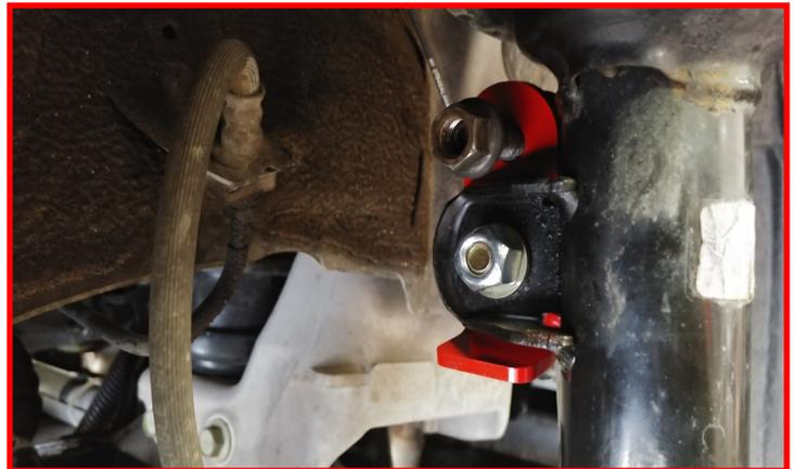
Install the front wheels and lower the vehicle to the ground. Torque the lug nuts to the wheel manufacturers specs. Jounce the front end to settle the suspension. Torque the upper strut spacer to **30 ft-lbs**.
