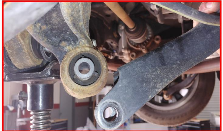
Loosen but do not remove the **lower control arm** bolt at the subframe. Remove the **lower strut bolt** on the lower control arm and the **control arm bolt** at the knuckle.
