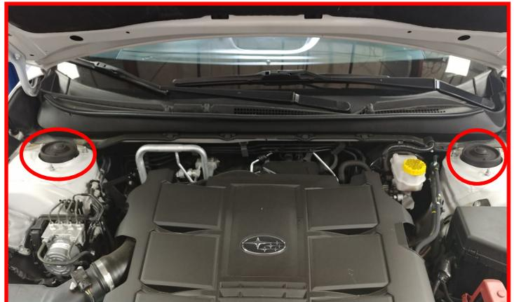
Locate the ReadyLIFT front strut extension. These are driver and passenger side specific. Passenger side shown. Install to the top of the strut using the **factory hardware**. Torque to **30 ft-lbs**.
