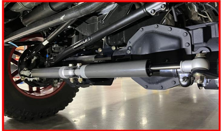
With all the hardware tightened and torqued to spec, complete a full lock to lock sweep of the steering to ensure there are no clearance issues, binding or bottoming out and/or over extension of the stabilizers.
