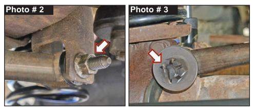
Remove cotter pin using pliers. Remove nut using a 1-1/8" socket \ wrench. (Photo # 3) Retain OEM hardware.
