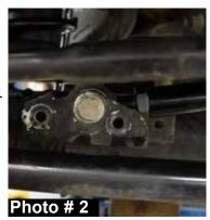
8. Place an adjustable wrench on the machine flat portion of the new Skyjacker adjustable front track bar & tighten the jam nut of the new Skyjacker rod end using an adjustable wrench.
