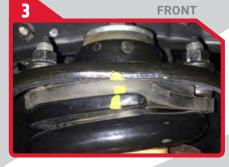
Before removing the strut assemblies mark the coil spring, spring isolator and strut tower to ensure the spring is reinstalled correctly.
