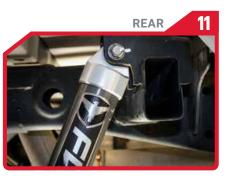
Orient the passenger side reservoir to the rear with the roost guard facing to the front
