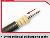
Orient and install the bump stop on the shock shaft as shown.
