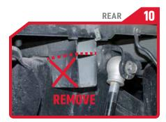
• Use a body saw, cutting wheel, or Sawzall to remove the bed locating tab to provide clearance for the Falcon Shock reservoir.
