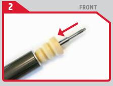
Orient and install the bump stop onto the shock shaft as shown.
