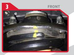
Before removing the strut assemblies mark the coil spring, spring isolator and strut tower to ensure the spring is reinstalled correctly. The spring must be reinstalled in the same orientation that it was removed.
