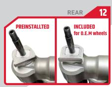
Make sure the correct alignment tab is installed on the Falcon Shocks.
