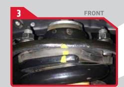
Before removing the strut assemblies mark the coil spring, spring isolator and strut tower to ensure the spring is reinstalled correctly. The spring must be reinstalled in the same orientation that it was removed.
