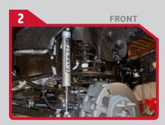
· Install the front shocks with the shaft down.
