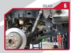
Install the rear shocks with the shaft
