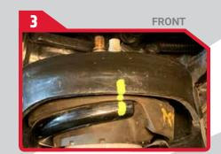
Before removing the strut assemblies mark the coil spring, spring isolator and strut tower to ensure the spring is reinstalled correctly.
