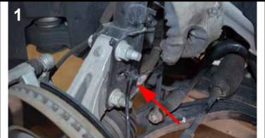
Raise vehicle on jack stands and remove wheels. Disconnect the ABS and brake hose.
