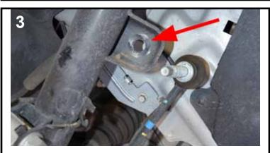
Disconnect sway bar end link from strut.
