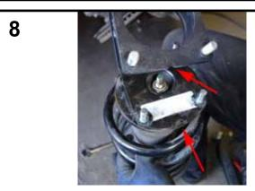
Install spacer on strut using factory nuts. Align notched edge with curved edge of strut mount. Reinstall in vehicle with curved edge facing away from engine.
