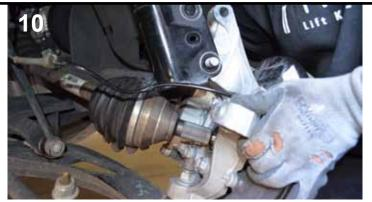
Reinstall lower strut mounting bolts while guiding axle through the spindle. Tighten all strut nuts fully, upper and lower.
