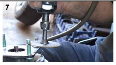
Cut 0.25" from the top of the mounting studs on the upper strut.
