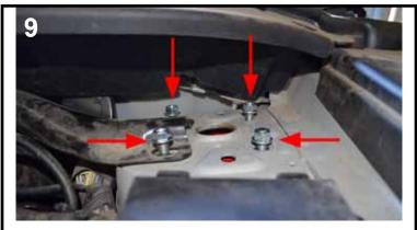
Reinstall upper strut mounting nuts. Do not tighten fully.
