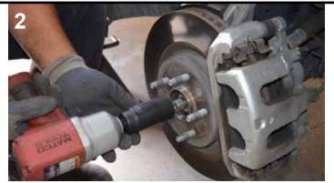
Loosen & remove the axle nut, and push the axle through the spindle.
