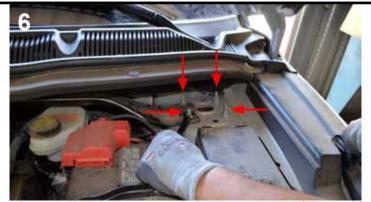
Remove nuts from upper strut mount. Support weight of strut before removing final nut. Remove strut from vehicle.
