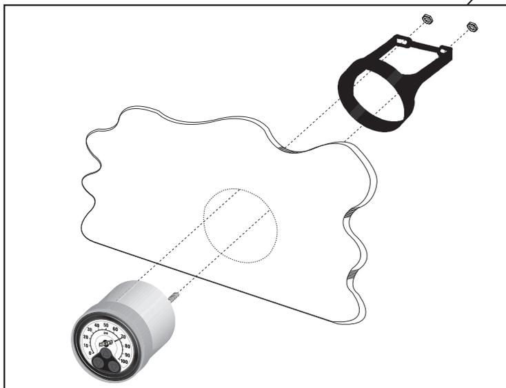
fig. 6 Optional Dashboard Mounting (Exploded View)
