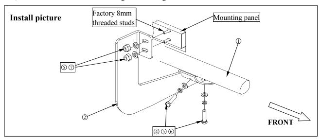
Step 4: After checking for proper clearance and alignment of the side bar on the vehicle, fully tighten all hardware.
