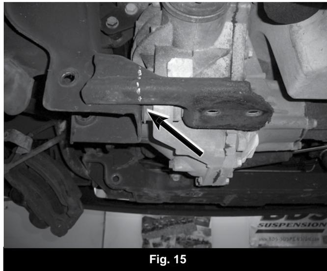
32. Support the front differential with an appropriate jack. Remove the differential mounting hardware and lower the differential from the vehicle and set aside. Save hardware.
