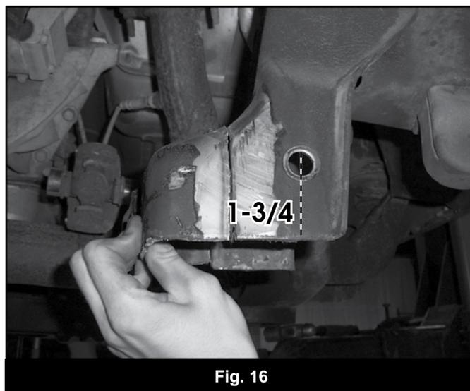
34. Using a reciprocating saw (recommended), hack saw or cut-off wheel, cut the pocket along cut lines.
