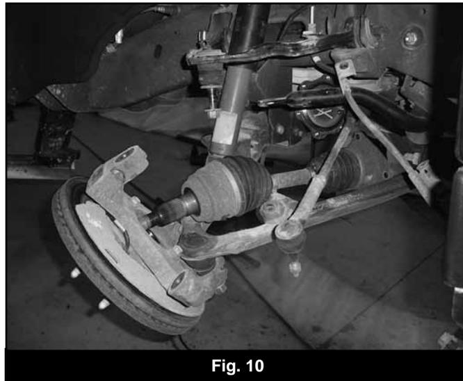
22. Remove the lower ball joint nut and thread back on by hand one or two turns. Strike the knuckle near the ball joint to release the taper. Remove the ball joint nut and remove the knuckle from the lower control arm. Save the lower ball joint nut and set the knuckle/hub assembly aside.
