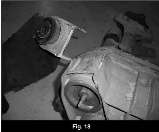
38. Install the provided large bushings (3624RB) and 0.750" OD x 2.950" long sleeve (15) into the eye of the new driver's side differential bracket (O1185).
