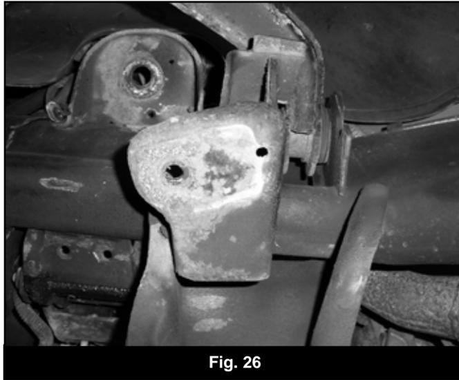
48. Locate the new provided bump stop brackets (02199). Place a bump stop bracket up to the original mount and line up the center of the two slots with the two holes in the factory mount. Using the third slot in the bracket as a guide, mark the center position to be drilled (Fig 27). Remove the bracket and drill a 7/16" hole at the mark.
