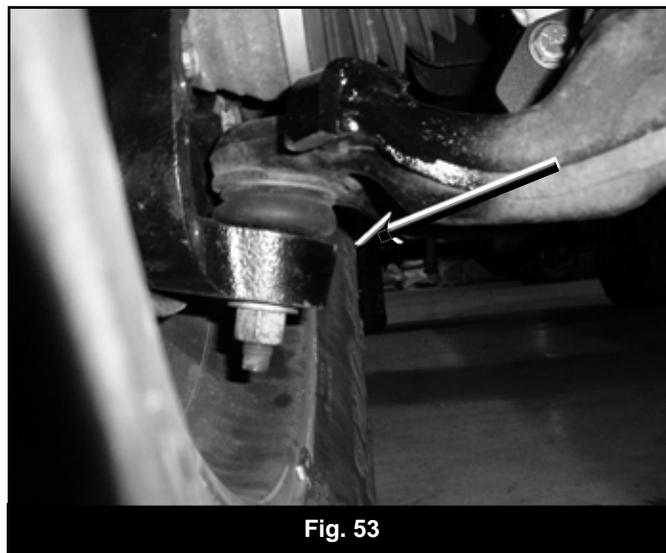
6. To determine the Z-height use the following equation:  $Y-X=Z$ . For the intended 7" of lift the value for Z should be approximately 4". If your value for 'Z' is less than 4" the torsion bars need to be adjusted up (tightened). If your value for 'Z' is more than 4" the torsion bars need to be adjusted down (loosened). These values are for reference but should not vary more than 1" in either direction.
