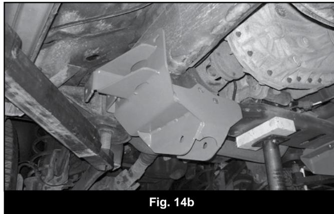
30. Remove the bracket and drill / clearance holes to 11/16". A step drill is highly recommended.
