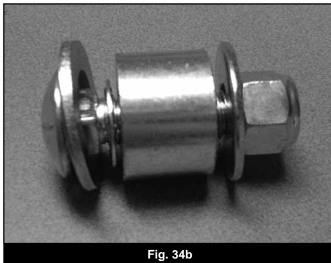
104. Install bumper onto vehicle with spacers over the carriage bolts. There are 2 bolts that will need to have a 3/4" washer added under the head. These bolts only go through one layer of the bumper. The rest of the bolts do not need a washer under the head of the carriage bolt.
