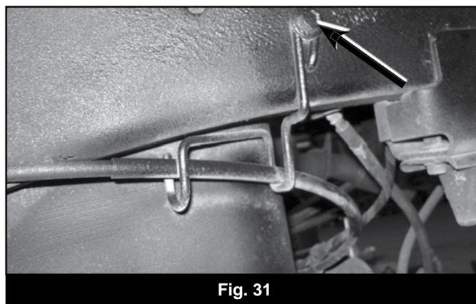
85. Disconnect the parking brake cable by unthreading nut with 13mm ratchet wrench.
