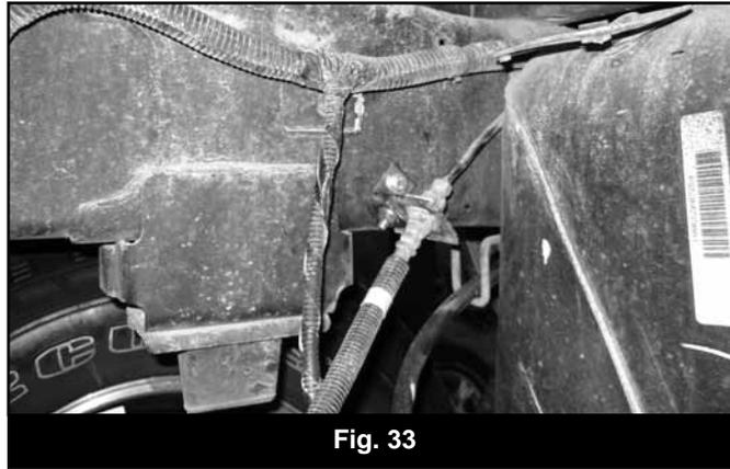
98. Attach 'L' bracket to the frame with 1/4"x1" Self threading bolt. Attach brakeline bracket to 'L' bracket with 1/4" x 1" hardware. Tighten to 15 ft-lbs. (#784).
