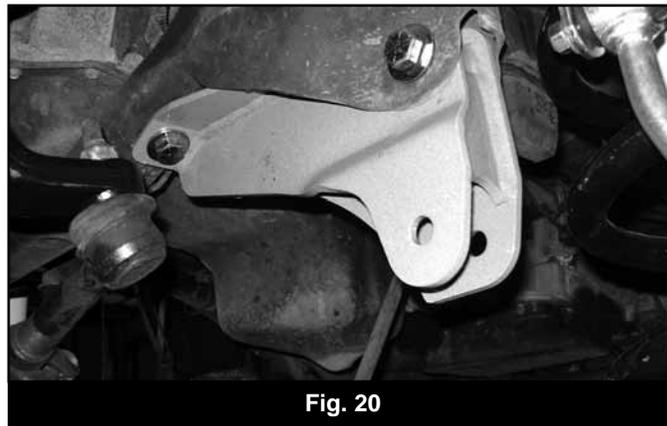
48. Tighten 9/16" hardware to 95 ft-lbs, 5/8" hardware to 120 ft-lbs.
