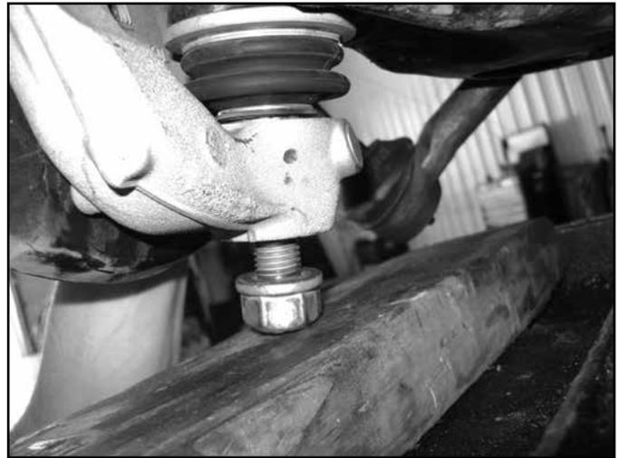
17. Remove the knuckle and hub assembly from the vehicle.
