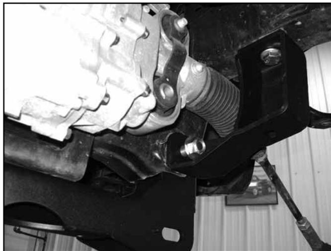
33. Install differential to the new drop brackets with 9/16" x 3-1/2" hardware (BP #681). (Fig 22a, 22b)
