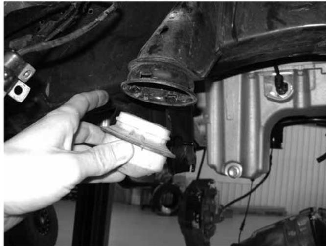
37. Clearance the hole inside the bump stop cup to 11/16", a step drill is highly recommended, if one is not available, a rotary die grinder can be used. Insert and seat 1/2" rivet nut. Follow rivet nut installation at the end of the instruction sheet. (Fig 25)
