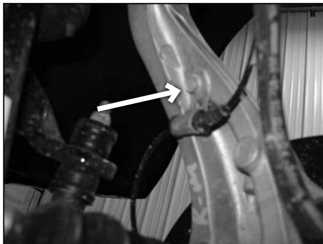
12. Remove the ABS sensor from the side of the knuckle (T30), retain mounting bolt. (Fig 5)
