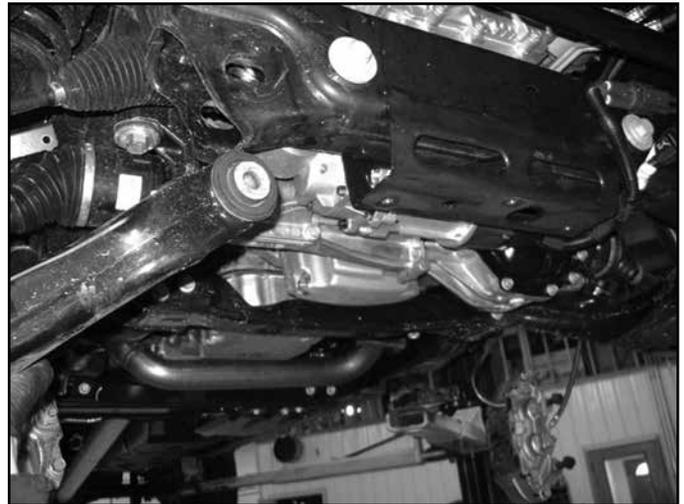
19. Remove the factory struts. Remove the lower bolt that attaches to the control arm and the 3 nuts that attach the strut to the upper strut mount. Do NOT remove the center nut that holds the strut assembly together.
