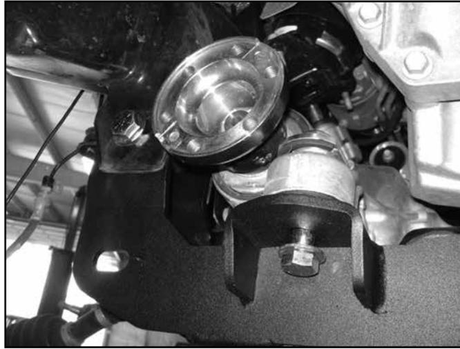
35. Reconnect the differential breather line and the central axle disconnect wiring harness.
