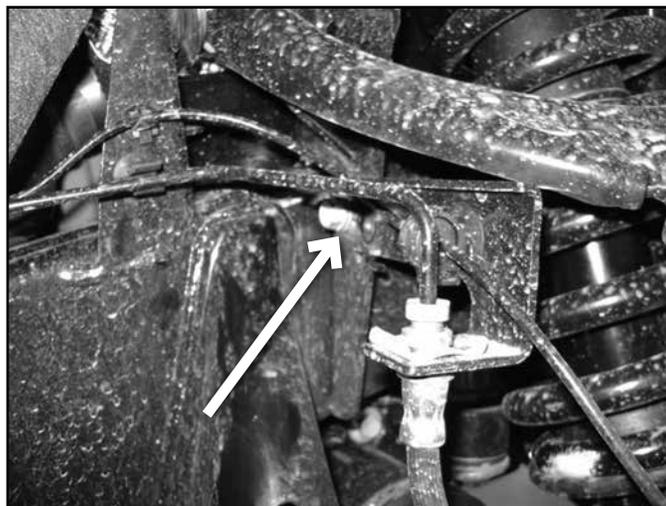
9. Disconnect the brake caliper from the steering knuckle, retain mounting bolts. Hang the caliper out of the way; do NOT allow the caliper to hang from the brake line. (Fig 2)
