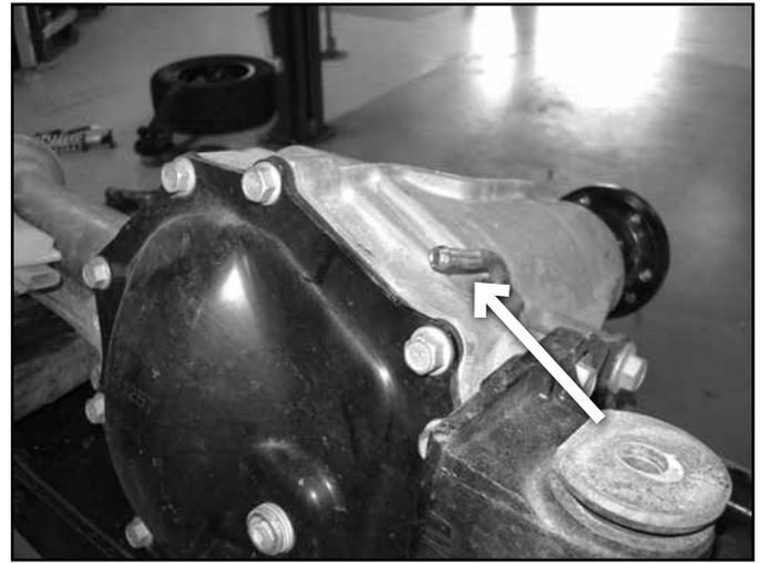
21. Disconnect the front drive shaft from the differential. Discard front mounting hardware, it will not be reused) (Fig 13). Disconnect the front driveshaft from the transfer case, *SAVE* hardware, it will be reused. Remove the front driveshaft from the vehicle.
