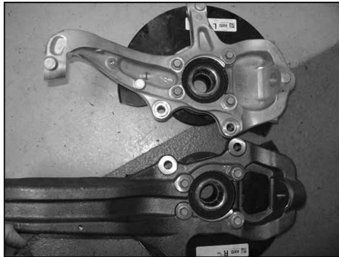
45. Apply loctite to the factory hub bolts, and tighten hub hardware to 133 ft-lbs.
