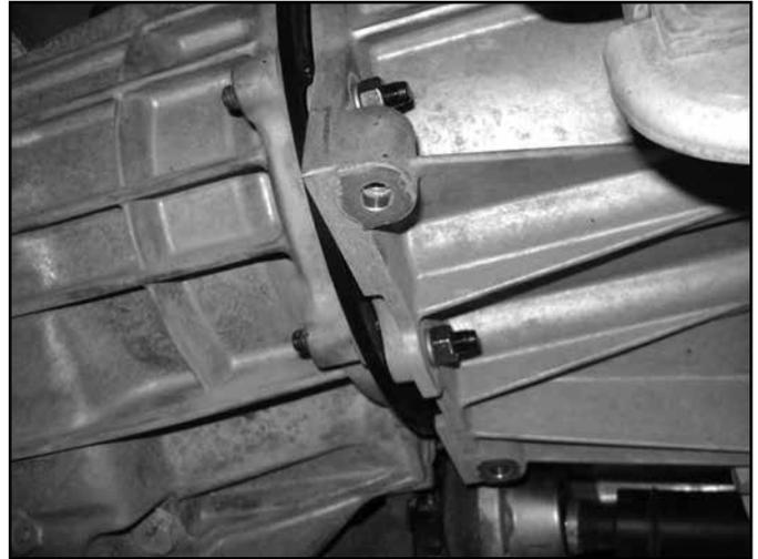
66. Reinstall transmission mount and crossmember with factory hardware, reattach wiring harness, and transfer case breather. Reinstall the rear driveshaft with factory straps and hardware. Tighten all hardware to factory specifications
