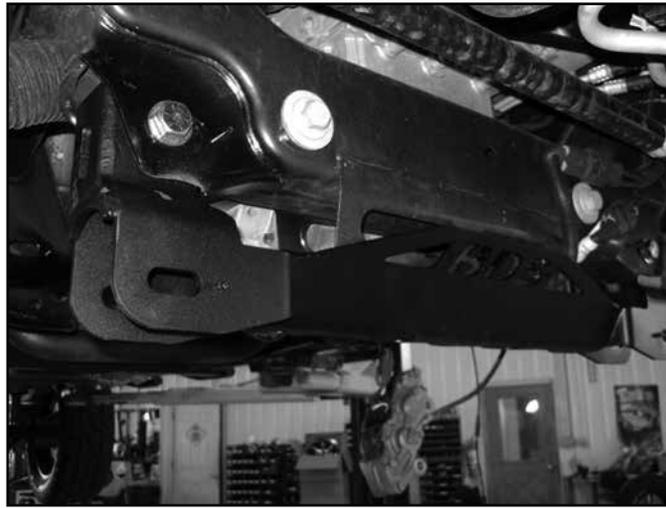
32. Install the new differential drop brackets (02809 – DRV, 02810 – PASS) with new 14mm x 30mm bolts and washers (BP #681) to the frame. Brackets will attach to the front cross member hardware, attach with 5/8" nuts and washers. Push the differential brackets all the way towards the front of the vehicle and tighten 14mm hardware to 95 ft-lbs. Leave 5/8" hardware loose. (Fig 21)
