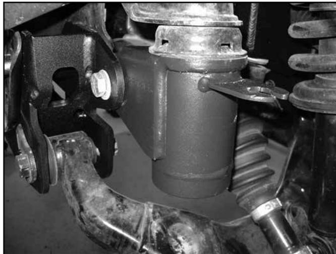
39. Install lower control arms with factory cam bolts and nuts. It is recommended to run the front bolts from Rear to Front, and the rear bolts from Front to Rear so that the nuts are easily accessible. They must be torqued to 170 ft-lbs later in the installation. Snug, but do not tighten at this time.
