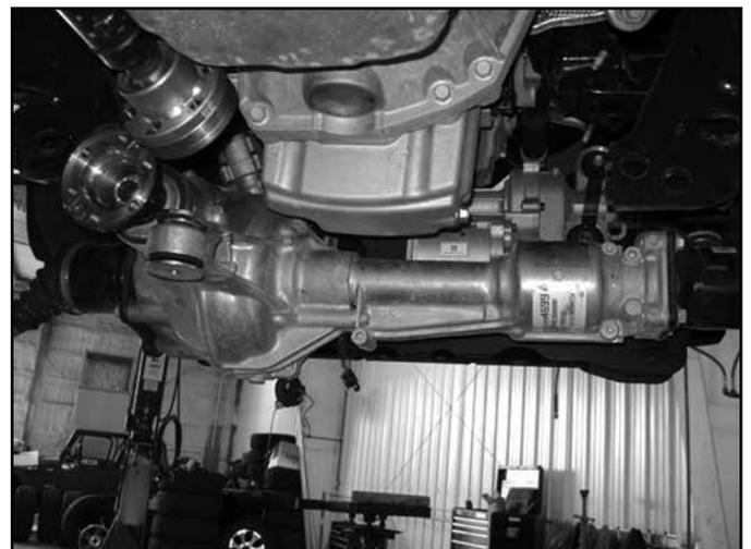
34. Raise the rear differential mount. Install rear cross member with new 5/8" x 4-1/2" hardware (BP #680). Attach differential to rear crossmember with new 9/16" x 3-1/2" hardware (BP#681). (Fig 23)
