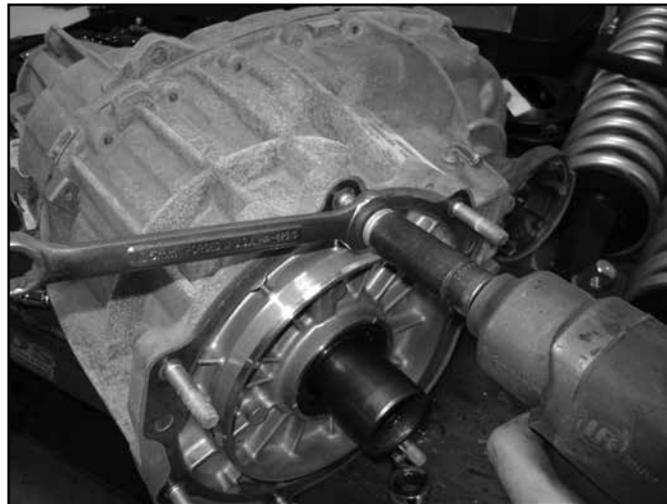
64. Install new index ring assembly with loctite on the new 10mm Flat Head Allen Bolts (BP #827), leave the factory gasket on the transfer case. Tighten to 35 ft-lbs (Fig 40a).
