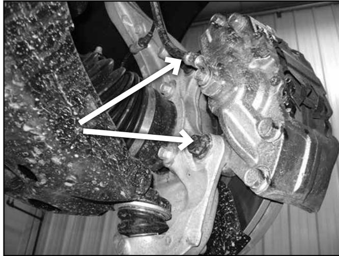
10. Remove the torx head bolt (T30) that attaches the rotor to the hub. Keep bolt for reinstallation. (Fig 3)
