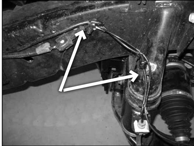
55. Zip tie the ABS wires to the brakeline to allow adequate slack through wheel travel and turning motions.
