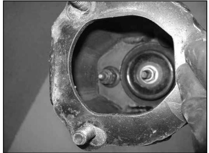
43. Install the strut and spacer into the vehicle. Attach the strut to the upper mount with new 3/8" nylock nuts and washers (BP #943). Attach lower mount to the lower control arm with factory bolts. Tighten the 3/8" hardware to 35 ft-lbs, do NOT tighten the lower mount at this time. It will be done at the end of the installation with the vehicle weight on the ground. (Fig 29a, 29b)
