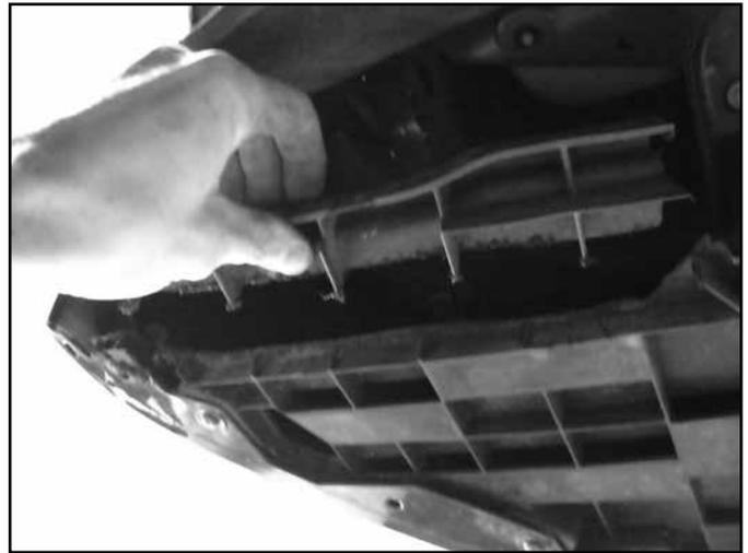
95. Remove the nut clips from the trimmed piece. Hold the inner fenderwell up to the front support piece and drill new holes for the mounting hardware at a convenient location. Attach the inner fender to the plastic support piece with factory torx bit hardware. Trim a slight amount on the plastic bumper cover for additional clearance if required. (Fig 51a, 51b)
