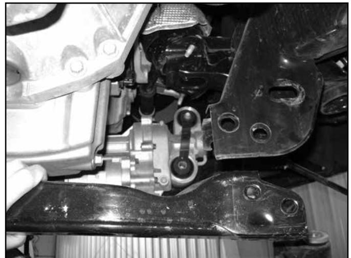
23. Support the differential with a hydraulic jack (transmission jack preferred). Remove the remaining two front mounting bolts and lower the differential from the vehicle. (Fig 16)
