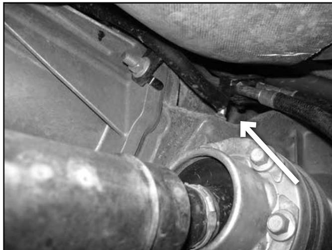
61. Support the transmission with a transmission jack, use extra care not to damage any surfaces on the transmission. Remove the factory transmission crossmember, remove the transmission mount, retain all hardware. (Fig 38a, 38b)
