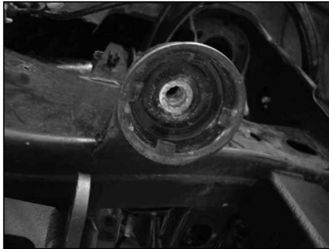
38. Attach the new bump stop extension (02813 – DRV, 02814 – PASS) to the rivet nut with  $\frac{1}{2}$ " x 2" hardware (use socket and extension to attach) and to the cross member with  $\frac{1}{2}$ " x 1-1/4" bolt, washers, and nut. (BP #683) (Fig 26)
