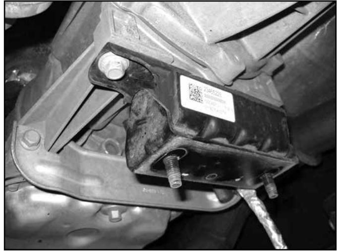
62. Support the transfer case. Remove the 7 nuts that hold the transfer case to the transmission and remove the transfer case from the vehicle.
