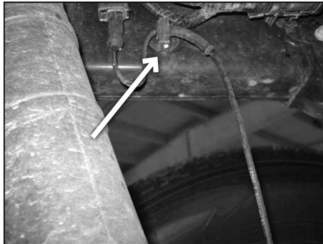
77. Remove the e-brake cable guide bracket from the side of the frame rail on the driver's side. It will not be reinstalled.
