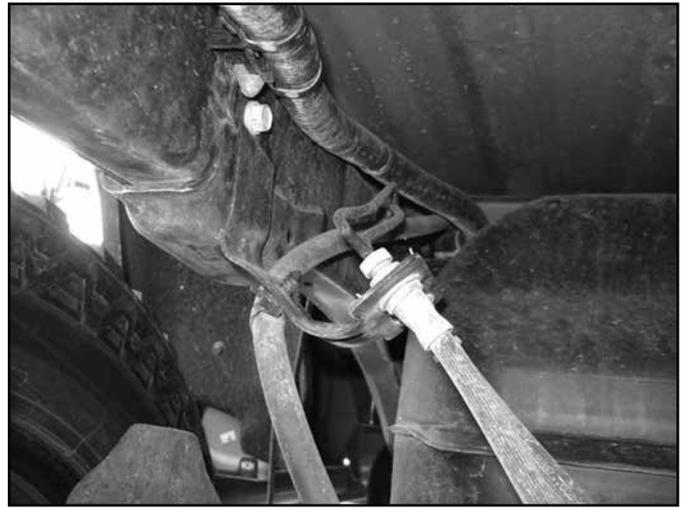
79. Working on one side of the vehicle at a time. Support the axle with a hydraulic jack, remove the factory u-bolts. Remove the stock shocks, retain hardware.
