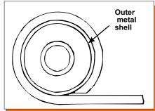
**Note:** When a sleeve is not used, apply a light coat of grease to the original shoulder bolt. **Remember:** Most spring eyes have an outer metal shell. Some shackles are this way as well. The outer shell must be removed.
