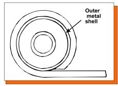
Note: When a sleeve is not used, apply a light coat of grease to the original shoulder bolt. Remember: Most spring eyes have an outer metal shell. Some shackles are this way as well. The outer shell must be removed.
