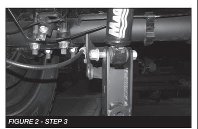
4. Locate the supplied 1/2" hardware. Rotate the shock 90 degrees and install the new bracket to the factory lower shock mount Torque to 90-lbs. SEE FIGURE 3
