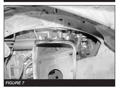
7. Install the FT825251 Coilover into the new upper mount using the ½-13 x 2-¼ bolt from the shock hardware. Torque 90 FT-LBS. **SEE FIGURES 8-10**
