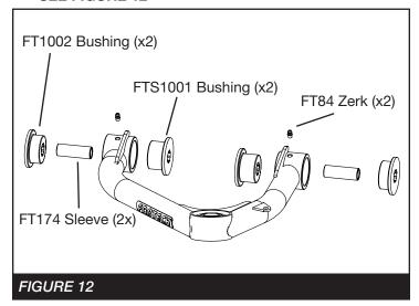
11. Install the upper arm using the factory hardware. Place the new FT58-1 washers on the inside and outside of the bushings. When installing the arm on the truck make sure the barrel gussets are up. Torque to 200 FT-LBS. SEE FIGURES 13-14
