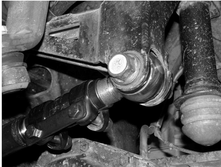
8. After the track bar is installed it may be necessary to a have vehicle Alignment preformed
