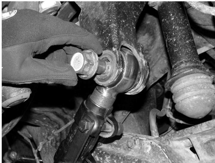
7. Center the axle accordingly using the adjuster sleeve in the on the track bar. After all adjustments have been made lock down the adjuster sleeve with the cross bolts. It is important that the sleeve is locked down with cross bolts perpendicular to the diff cover. **SEE PHOTO BELOW**
