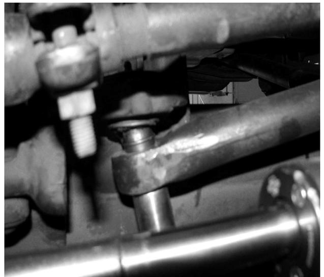
5. Install the New Fabtech adjustable Track Bar first at the lower pivot using thread lock and the factory nut. Tighten the nut to 183 ft-lbs. **SEE PHOTO BELOW**
