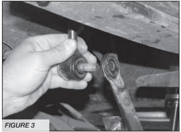
Locate the one FT30476 sway bar link, four FT1004 bushings, and two FT50089 sleeves. Press the bushings and sleeves into the barrels on the sway bar links.
