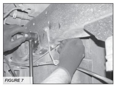
Mount the lower end of the link to the sway bar one ½-13 x 2-1/2 bolt, two ½"washers and one c lock nut. Torque to 90ft-lbs. SEE FIGURE 8
