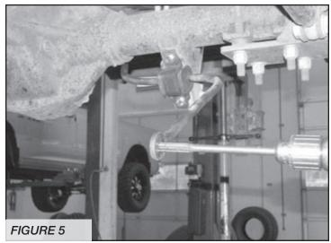
Locate the FT30475 nut tab, one ½"-13 x 2-1/2" bolt and a ½" washer. Mount the link to the frame using the hardware listed above. Torque to 90ft-lbs.
