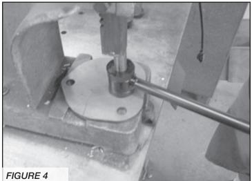
5. Using a ½" drill bit, drill out the sway bar to ½". **SEE FIGURE 5**
