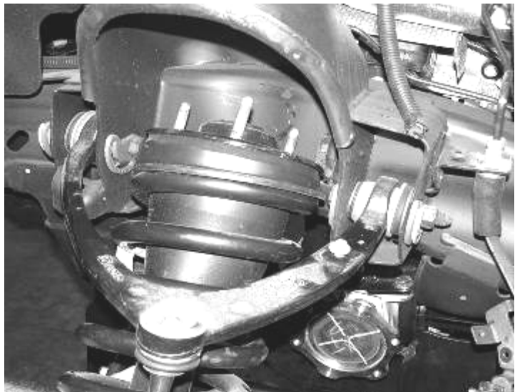
19. Locate the factory upper shock hardware. Install the shock into the factory shock bucket and leave loose. SEE PHOTO BELOW.
