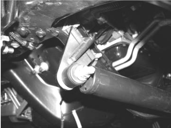
Picture Shown with Factory Stabilizer re-installed
