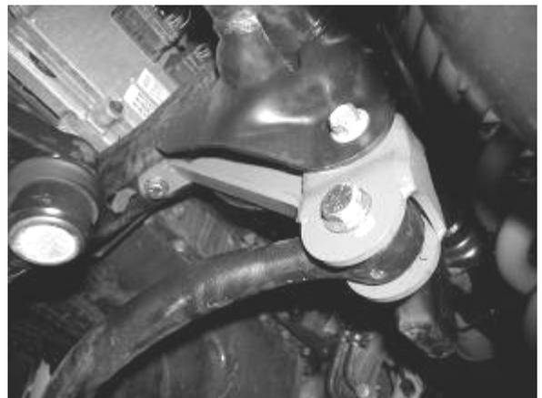
16. Connect the drag link to the new drop pitman arm. Torque the original nut to 45 ft-lbs. SEE PHOTO BELOW.
