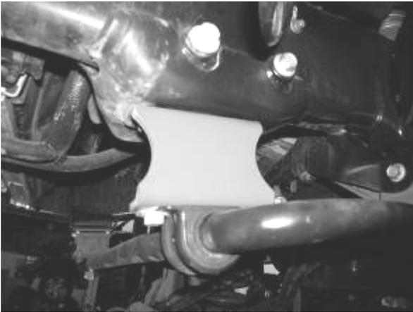
18. Attach the brake line tab back to the original mount using the original hardware. You may need to pull the factory hose through the bracket to gain some slack. Repeat this on the opposite side of the truck.
