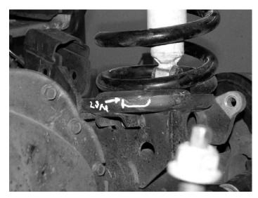
15. Connect the track bar to the new drop bracket using the supplied 9/16" x 3" bolt, nut, and washers. **NOTE: This may need to be done when the truck is back on the ground.** SEE PHOTO BELOW.
