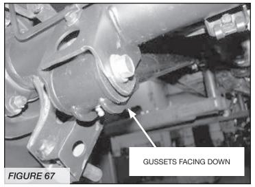
46. Remove the driver upper link and install an assembled Fabtech link with the gusset facing upward in the frame pocket and down at the axle mount with the stock hardware. Repeat on the passenger upper link.
