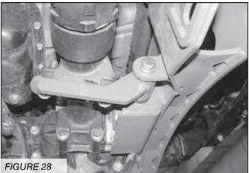
21. Locate the Fabtech rear crossmember FT70052 06-09 models FT70163 10-12 models, with the supplied 9/16"x5 bolts, nuts, and washers install the crossmember to the factory control arm pockets. Leave loose at this time. Re-install the factory rear differential nut at this time. **SEE FIGURE 29**
