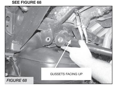
47. Working from the driver side, locate FT70086 Rear Coil Spacers and the supplied 3/8" & 8mm hardware. Position the coil spacer up into the coil bucket on the frame and attach to the factory bumpstop mount with the 8mm hardware (only tighten enough to hold the spacer in position). Mark the three holes in the spacer to the coil bucket and remove the spacer. **SEE FIGURES 69-70**
