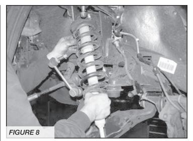
Remove and save the factory lower control arms with the hardware.
