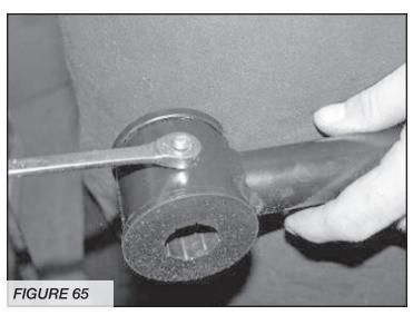
45. Remove the driver lower link and install an assembled Fabtech link with the gussets facing down using the stock hardware. Repeat on the passenger lower link.
