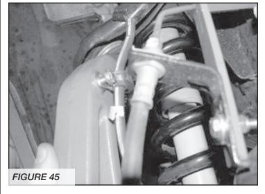
33. Now attach the tie rod ends with the factory castle nut and supplied cotter pin. (torque the tie rod ends to 70 ft. lbs.)
