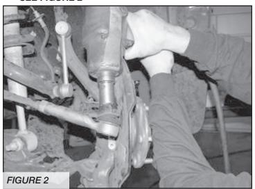
Remove the sway bar end links from the factory steering knuckles and leave connected to the bar. Then remove the bar from the truck. Save the bar and end links with all hardware. SEE FIGURES 3-4
