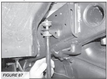
56. Locate the supplied 12mm bolt, nut, and large washers. Place a washer onto the bolt and insert into the sway bar from the inside of the bar. Follow with another large washer. Mount the bar to link and follow with another large washer and the C-lock nut. Tighten the lower bolt first and then the upper nut. Only tighten enough to get the bushings to bulge. **SEE FIGURE 88**
