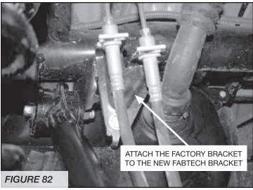
53. Re-connect the ABS sensor to the harness. Locate the ABS bracket on the crossmember and carefully bend the bracket down (do not over bend, it could brake the bracket) just enough so it lines up with the clamp on the ABS lines. Check to ensure that there will be enough slack for the cables during suspension cycling. Attach the ABS clamp to the bracket with the factory hardware.
