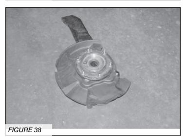
28. Support the lower arm with a floor jack and install the new assembled steering knuckle to the lower ball joint with the factory castle nut and supplied cotter pin. Raise the jack enough to locate the knuckle up into the upper ball joint (pull down on upper arm) and attach with the factory castle nut and supplied new cotter pin. Upper ball joint torque 81ft-lbs. Lower ball joint 103 ft-lbs.
