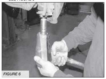
10. Remove the three upper nuts from the top of the strut assembly then the lower bolt from the strut at the lower control arm. Remove the shock assembly as one complete unit and save with the hardware if installing the Basic Kit (coil spacer) retain shock assembly, if installing Dirt Logic coilovers discard shock assembly.
