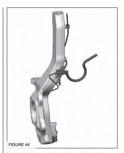
32. Install brake rotors & brake calipers with the factory hardware and thread lock compound. Route the ABS onto backside of the steering knuckle. There should be enough slack just inside the wheel well to pull the line down for the factory sensor to bolt into the new Fabtech steering Knuckle. Using the supplied adel clamps and the ½" x ¾" bolts, washers, & split washers, reinstall the factory ABS Sensor into the Fabtech Knuckle. **SEE FIGURES 45-46**
