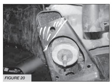
17. Use a sawzall and cut the marked area from the mount. Next, sand and clean the cut area on the mount. Locate FT70094 Weld-in Plate. Check fit the plate against the mount for proper fitment (it may be necessary to sand the mount for proper fitment of the plate). Weld the plate in and paint after it has cooled. SEE FIGURES 21-24
