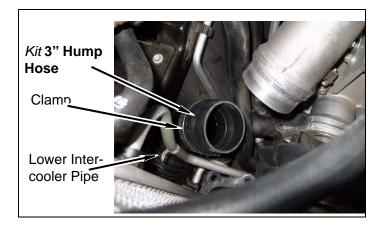
c. Place factory clamp on hump hose. Install factory elbow on intake housing and rotate factory elbow into the *kit* **3**" **Hump Hose**.
