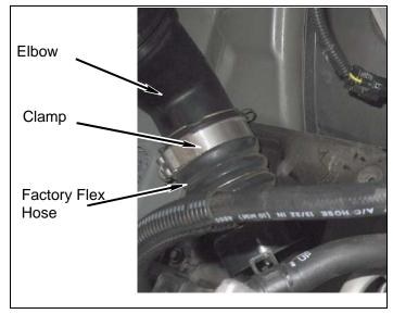
b. Install *kit* **3" Hump Hose** on lower intercooler pipe using factory clamp.
