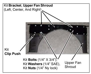
i. Using kit bracket, upper fan shroud (center) as template, drill two 1/4" holes in fan shroud lip. Install kit bracket, upper fan shroud (center) on upper fan shroud lip with two kit clips push.
