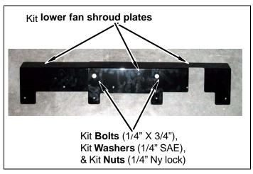
h. Install *kit* **lower fan shroud plates** (assembly) on core support with two kit **bolts** (1/4" x 3/4"), four kit **washers** (1/4" SAE), and two kit **nuts** (1/4" nylock). Using fan shroud plates as template, mark and drill two 1/4" holes in core support as shown. Install two kit push clips in the drilled holes.
