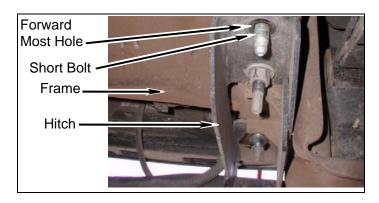
n. Install kit brackets (rear bumper) and hitch on frame with two long bolts, two kit washers (1-1/2 x 2-1/2 rectangular), two kit washers (14mm), into two kit nuts (14mm nylock).
