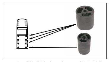
Install kit lift blocks on frame and bed with four kit bolts (12mm-1.75 x 100mm) and four kit washers (7/16" USS). Do not tighten.
