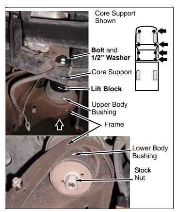
c. Install three kit lift **blocks** (with 5/8" hole) under body and on top of top body bushings, frame, and lower bushings, with three kit **bolts** (14mm-2.0 x 180mm) and kit **washers** (14 mm). Do not tighten.
