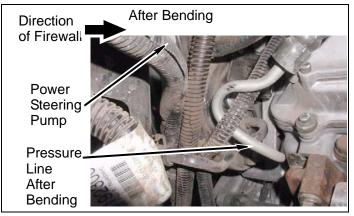
d. Carefully bend power assist pressure line up toward hood, to clear accumulator on brake hydro boost.
