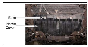
Remove plastic cover from push clip, lower radiator hose and vehicle.
