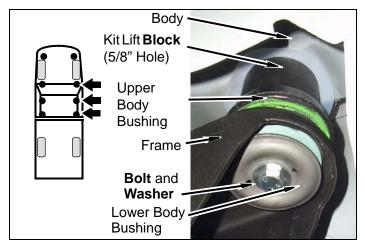
d. Lower cab onto kit lift blocks.
