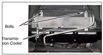
c. If necessary, carefully bend hard line and secure with kit **zip tie**.
