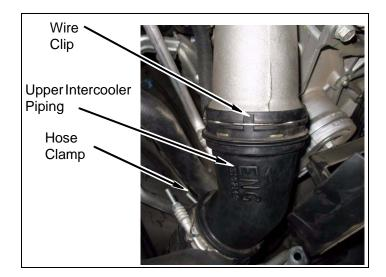
b. Remove intercooler pipe and hose from vehicle
