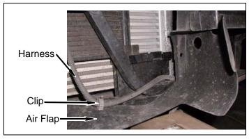
e. Remove two clips, three push pins, and air flap from core support.
