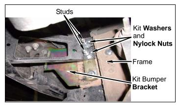
h. **3" kit passenger side:** Install kit **bracket** (3-stud), outer bumper brace, and kit **bracket** (rear bumper) on frame with a kit **bolt** (1/2" X 1 1/2") three kit **washers** (1/2" USS), and two kit **nuts** (1/2" nylock). Do not tighten.
