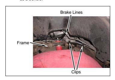
e. If possible, install harness in clip on frame driver side.
