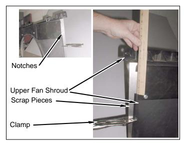
g. Using three kit **brackets**, **upper fan shroud** (left, center, and right) as templates, drill 1/4" holes in fan shroud.
