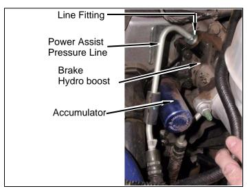
g. Remove bolt, clamp, and power assist pressure line from frame.
