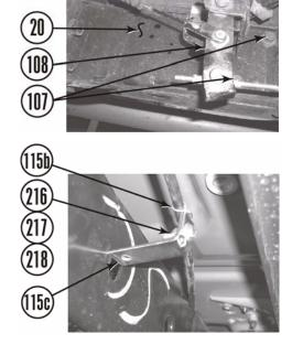
b. Install *kit* bracket (115c) on frame (20) driver side with bolt (115a).
