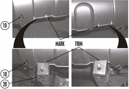
f. Position front outer bumper (10) on vehicle and install on front fenders (17), lower crush zone (11), core support (14), and side front outer bumper brace (19) with four screws (9 and 16), six push clips (13), six plastic bolts (12) and four bolts (15 and 18).
