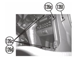
e. Position shift lever console (126a) on storage console (126b) and if applicable, install manual shift knobs (123 and 124) on manual shift levers (125 and 126).
