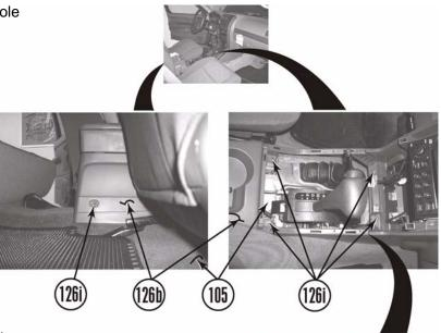
f. Lift storage console (126b) and locking clips (126j) from dash (126f).
