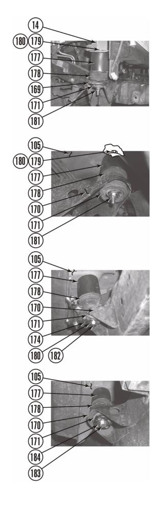
6. Install the bed passenger side spacer blocks.
