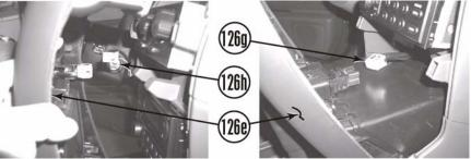
d. Install dash console cover (126e) on dash (126f) with four screws (126c) and four clips (126d).
