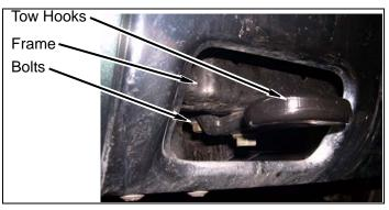
d. Remove four bolts and two side impact braces from frame.
