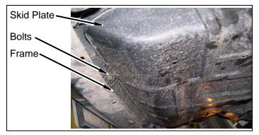
c. If equipped, remove four bolts and two tow hooks from frame.
