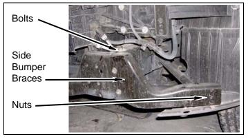
h. Remove four bolts and two side impact braces from frame.
