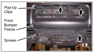
c. Remove six screws from driver and passenger front bumper fascia and wheel wells.
