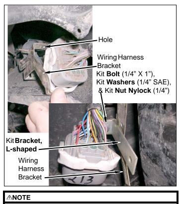
It maybe necessary to slightly bend tab on the back side of wiring harness bracket to fit over the top of the frame. b. Install wiring harness bracket and kit **bracket**, L-**shaped** on frame with bolt.
