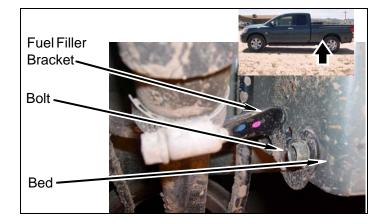
b. Remove fuel cap from fuel filler. Push fuel filler rubber gasket and fuel filler toward inside of bed.
