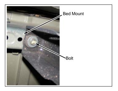
2. Remove three bolts, washers, and small bushing from three bed mounts on passenger side.
