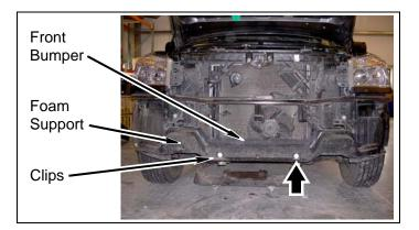
g. Remove six bolts, four nuts, and two side bumper braces from front bumper and side impact braces.
