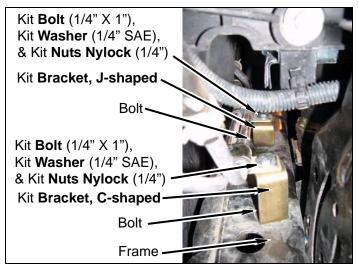
c. Install wiring harness on frame with kit zip-tie.
