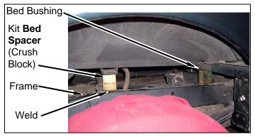
3. Tack-weld four kit **bed spacers** (crush blocks) to frame.
