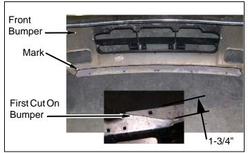
d. Cut front bumper where marked as shown.
