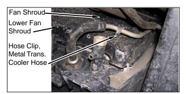
b. Remove transmission cooler hose and lower fan shroud from fan shroud and vehicle.
