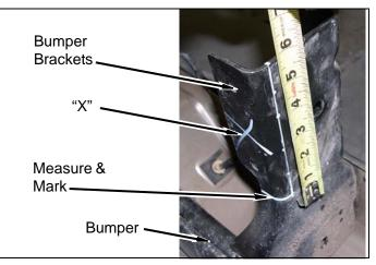
c. Cut and remove area of rear bumper brackets marked with an "X" where shown.
