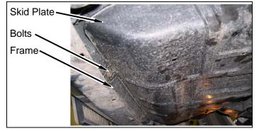
m. Mark and drill two 1/4" holes into skid plate. Install front bumper fascia straps onto skid plate with two kit **push clips**.
