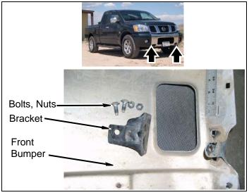
b. Position front bumper on front bumper brackets and visually inspect and the frame cross member where interference occurs along the bottom edge of the front bumper.
