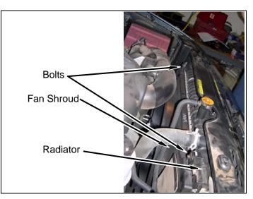
c. Install upper radiator hose on radiator with hose clamp.
