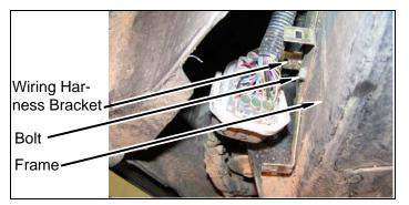
c. Remove two wiring harness push clips and wiring harness from frame / body mount perch.
