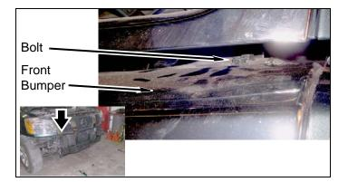
j. Install front bumper and two kit **spacers** on front bumper brackets with two kit **bolts** (M8-1.25 X 40mm). Do not tighten.
