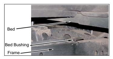
2. Install four bed bushings on four kit **bed spacers** (crush blocks). Position four kit **bed spacers** (crush blocks) on frame rail as shown.
