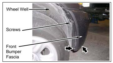
d. Pull driver and passenger wheel well back and remove four bolts from front bumper fascia and front fenders.
