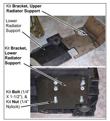
e. Position and mark holes from kit bracket, upper backing plate on side support as shown. Drill 1/ 4" holes where marked.
