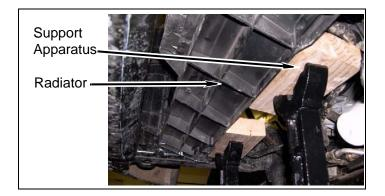
b. Mark and cut lower radiator support and ribs as shown.
