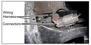
d. Remove two license plate light connectors from rear bumper.
