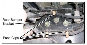
c. Disconnect two wiring harness connectors from wiring harness.
