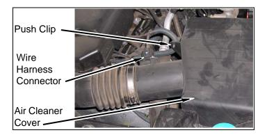
b. Remove two clips, hose clamp, and air cleaner cover from air cleaner base.
