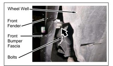
e. Remove six bolts and front bumper fascia from vehicle.
