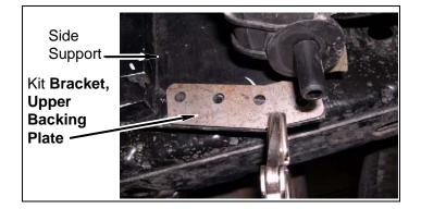
f. Install lower radiator support assembly and kit **bracket**, **upper backing Plate** on side supports with six kit **bolts** (1/4" x 1"), twelve kit **washers** (1/4" SAE), and six kit **nuts** (1/4" nylock).
