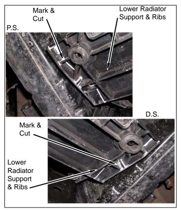
c. Position and mark twelve holes from kit **brackets, upper radiator support** on lower radiator support. Drill 1/4" holes where marked.
