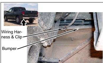
a. Remove wiring harness and clip from bumper.
