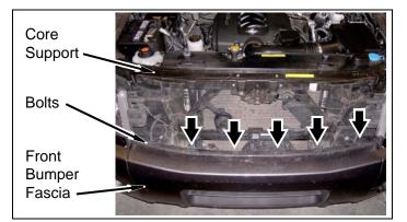
g. Install front bumper fascia onto support with three pop-up clips.
