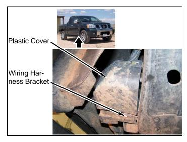
b. Remove bolt and wiring harness bracket from frame.
