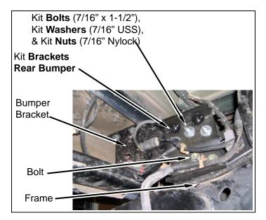
h. Install kit **bracket**, **hitch support** on hitch and rear bumper with four kit **bolts** (7/16" x 1-1/2"), eight kit **washers** (7/16" SAE), and four kit **nuts** (7/16" nylock).
