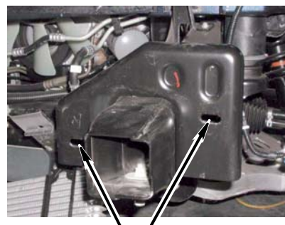
Remove the bumper mounting nuts from behind the frame flange
