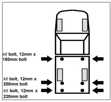
2. Repeat previous step on opposite side of vehicle. Tighten all *kit* **body mount bolts** at this time.
