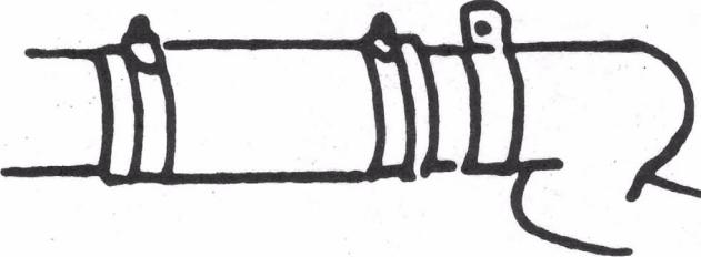
2. Ensure ample slack (approximately height of lift) in all brake lines, wiring harnesses, radiator and A/C hoses, window washer hoses, park brake cables, etc. before lifting bed.
