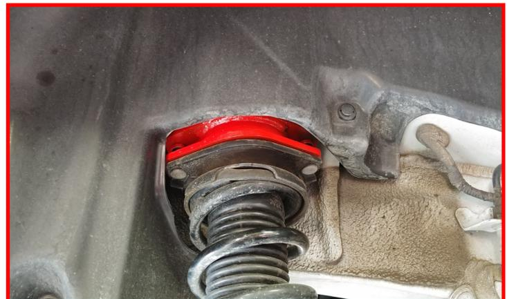
Raise the lower control arm into place and install the **lower strut hardware**. Do not tighten at this time. Use the jack and raise the lower control up to set pre load on the strut. Install the lower **knuckle bolt**.
