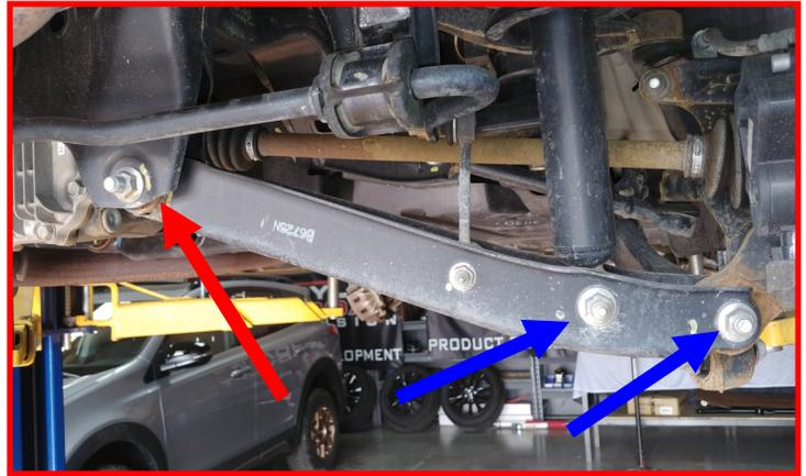
Lower the control arm down and remove the strut from the vehicle and let the control arm hang.
