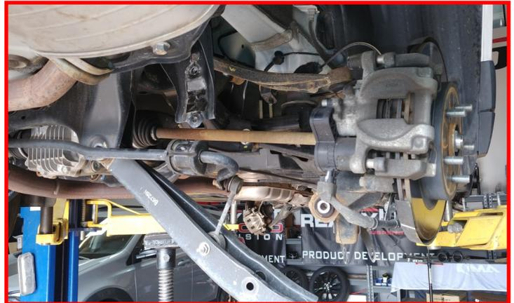
Install the ReadyLIFT strut extension using the **factory hardware**. You will have to start each nut before tightening fully. Run each nut down in an alternating pattern until you can torque them down. Torque to **30 ft-lbs**.
