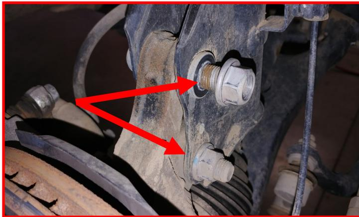
Remove the upper strut hardware. Make sure to hold the strut assembly from falling out of the vehicle. A helper is recommended for removal.
