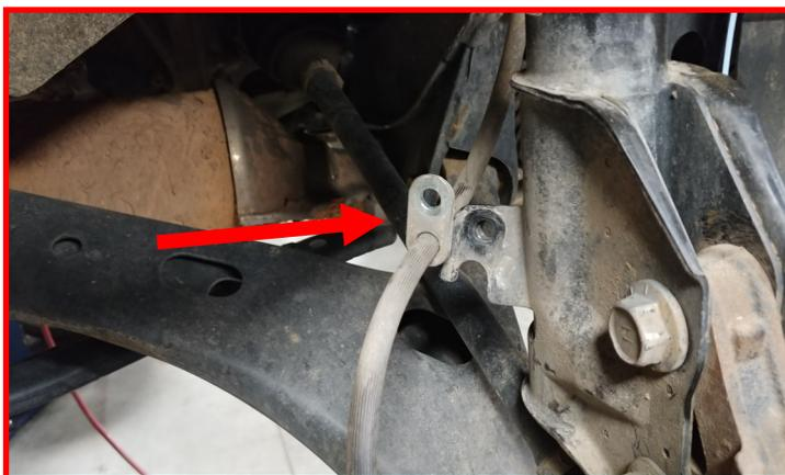
Reinstall the ABS clip back to the strut.
