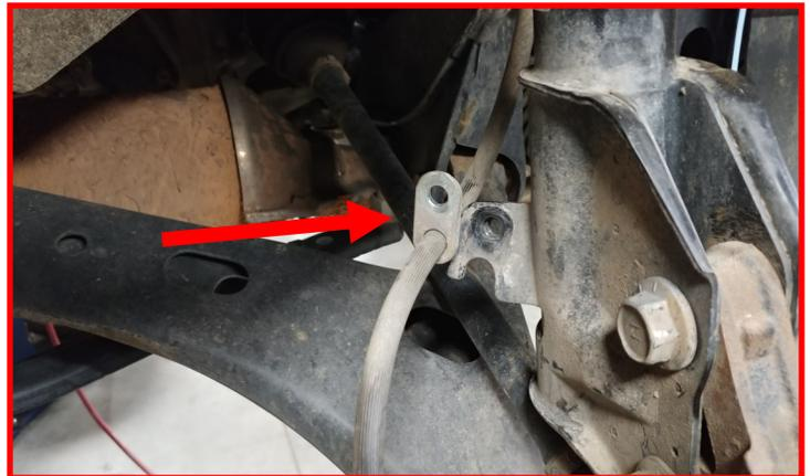
Remove the ABS wire from the strut body. Let hang out of the way.
