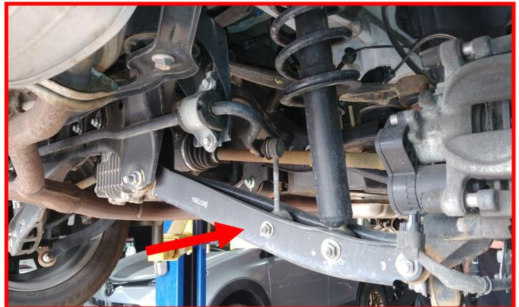
Remove the sway bar at the subframe and let hang out of the way.
