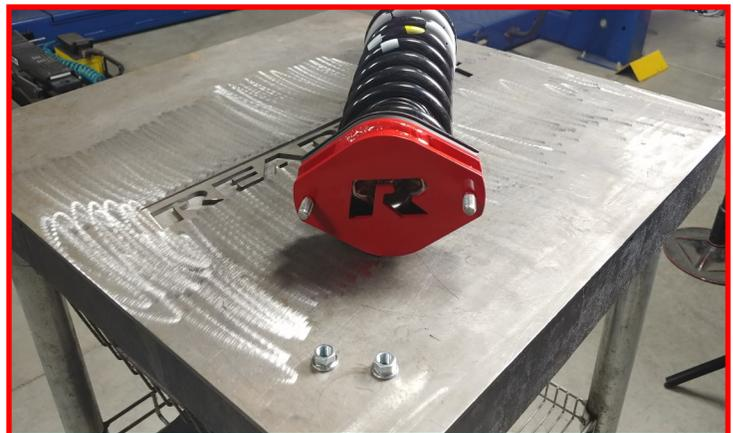
Install the completed strut assembly to the car using the provided **M10 flange nuts**. Do not tighten at this time. A helper is recommended.
