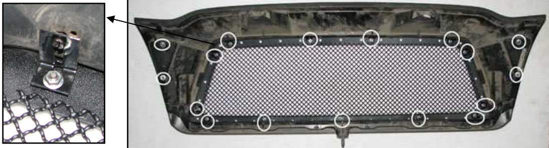
Figure 3 – Rear view of vehicle's shell; Grills attached with Metal Brackets and Flange Nuts
