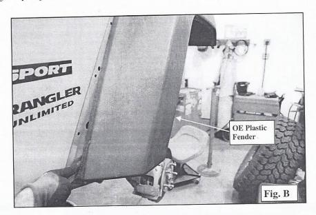
Step 5: Remove the OE plastic front inner fender liner from the vehicle.
