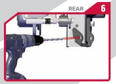
• Drill outside tab only using a 5/8" drill bit Using the softest setting to make the
