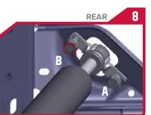
· B] Loosely install remaining bolt
