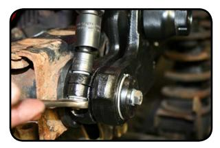
14. Tighten the spacer bolts using a 3/16" allen.
