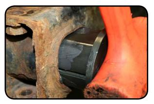
Grease the inside of the bushing and install the shaft. Make sure that the side with out splines at the end of the shaft is on the drivers side. Use a dead blow hammer if needed.
