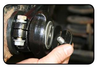
13. Torque the sway bar arm pinch bolts to 50 Ftlbs using a 9/16" socket and wrench.
