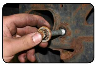
6. Install the busings into the cross member tube. The flat part of the busing needs to align with the flat part of the cross member tube. Use grease and a dead blow hammer to install the bushing.
