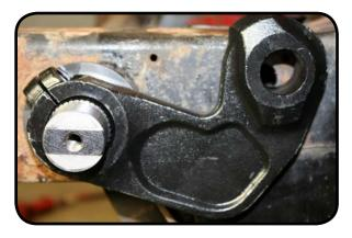
11. Install the drivers side sway bar arm. Use a dead blow hammer and drive it onto the smooth part of the shaft.
