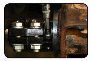
15. Install the locking knob using 1-1/2" wrench and blue treat locker.
