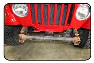
4. Check the cross member tube for any obstructions. Clean the tube using a barrel sander.
