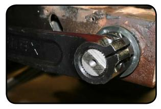
10. Install the locking arm on the drivers side. Make sure that it aligns with the passenger sway bar arm.
