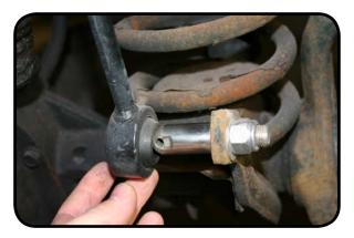
Remove the bolts from the sway bar mount using a 15mm socket or wrench. (Use tape to protect the paint.)
