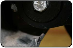
20. Reinstall the bumper. Use the two shorter bolts on the holes the align with the cross tube.
