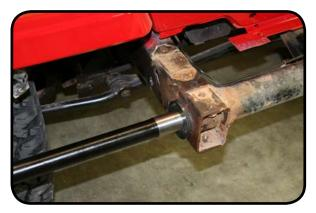
8. Install the spacer on the passenger side of the shaft. If needed use a chisel and hammer to open up the relief cut to install the spacer onto the shaft.
