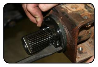
9. Install the passenger sway bar arm onto the shaft splines.
