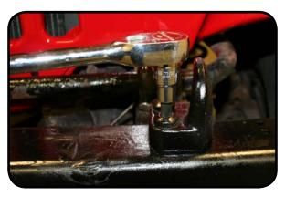
Remove sway bar links at the axle using an 18 mm socket (if using quick disconnects just slide them off the mount pin) Remove the pin or factory bolt.
