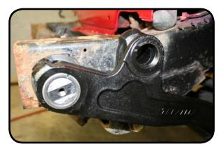
12. Install the end caps using 9/16" socket and blue tread locker. Torque to 20 Ft-lbs.
